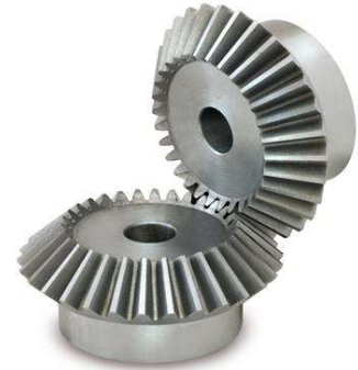
Type A Pressure angle 20° Ratio 1:1
